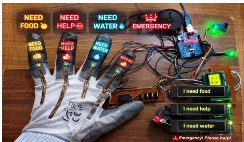
Figure 2: Output Of Smart Glove for Gesture to Speech Tranlsition
